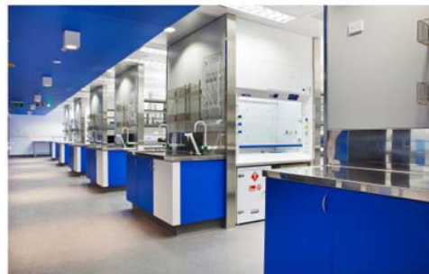
CARE IN POSITIONING SINKS AND FUME CUPBOARDS TO CONSOLIDATE SERVICES. THIS ALLOW TO MAXIMISE THE FLEXIBILITY IN THE CENTRE OF THE MODULE
