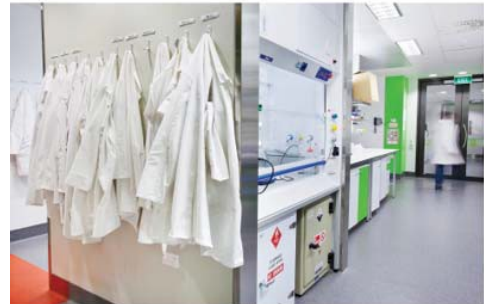
FUMECUPBOARD CENTRALISED TO CONCENTRATE HAZARDOUS WORK AND EFFICIENCY. BRINGING TOGETHER DG STORAGE
