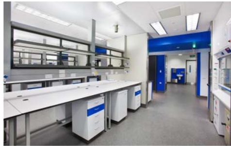
MODULAR, ULTRA MOBILE AND LOOSE BENCHING, UNDER BENCH STORAGE, REMOVABLE AND ADJUSTABLE SHELVING.
