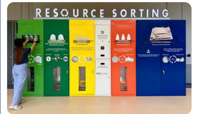
3 RSS with load cells and sensors to track collection of single-stream recyclables: PET bottles, HDPE containers, metal cans, glass, cardboard/ paper.
